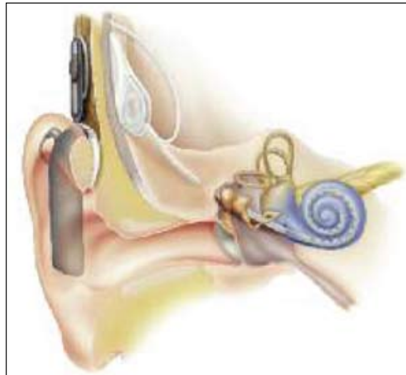
Figure 3: Diagram of the implanted multi-channel intra-cochlear electrode and receiver-stimulator unit of a cochlear implant.
